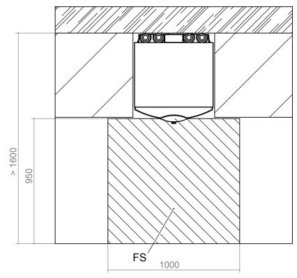
Key: DE819456a V3 Version 3 FS Free space for service purposes OKF Finished floor level All dimensions in mm.
