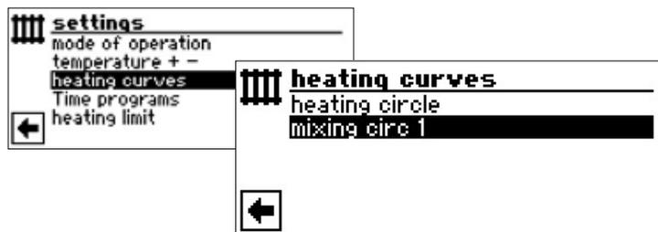
The screen changes to the menu "Heating curves Mixing circle 1". The heating curves can be programmed if no fixed temperature is defined.
