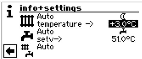
Finish entry by pressing the “rotary pushbutton”. This saves the required temperature. The program automatically activates the symbol
