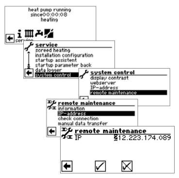
Enter the IP address of the remote maintenance server here
