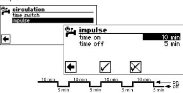
If the "Time off" setting is set to 0 minutes, the circulation pump will be switched on permanently during the released time periods.
