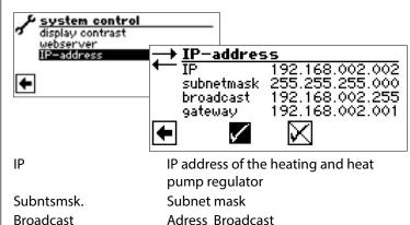
Gateway Gateway address of the connected router)
