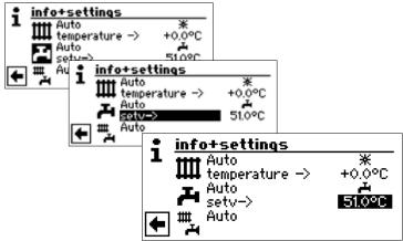
Set the required domestic hot water temperature (= setpoint value): 30 °C.
