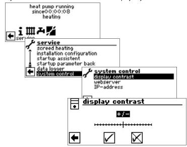
Adjust the contrast by turning the "rotary pushbutton"
