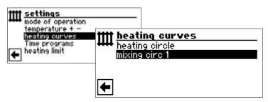
The screen changes to the menu "Heating curves Mixing circle 1". The heating curves can be programmed if no fixed temperature is defined.
